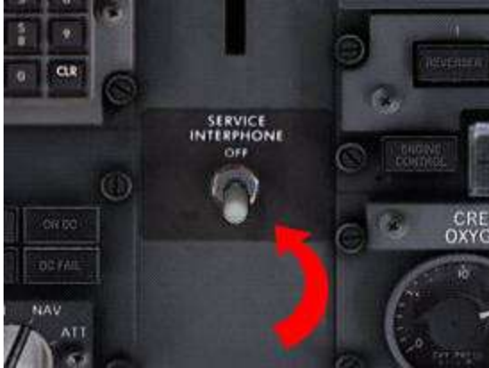
AFT OVERHEAD PANEL - ENSURE THE SERVICE INTERPHONE SWITCH IS SET TO 'ON'.
