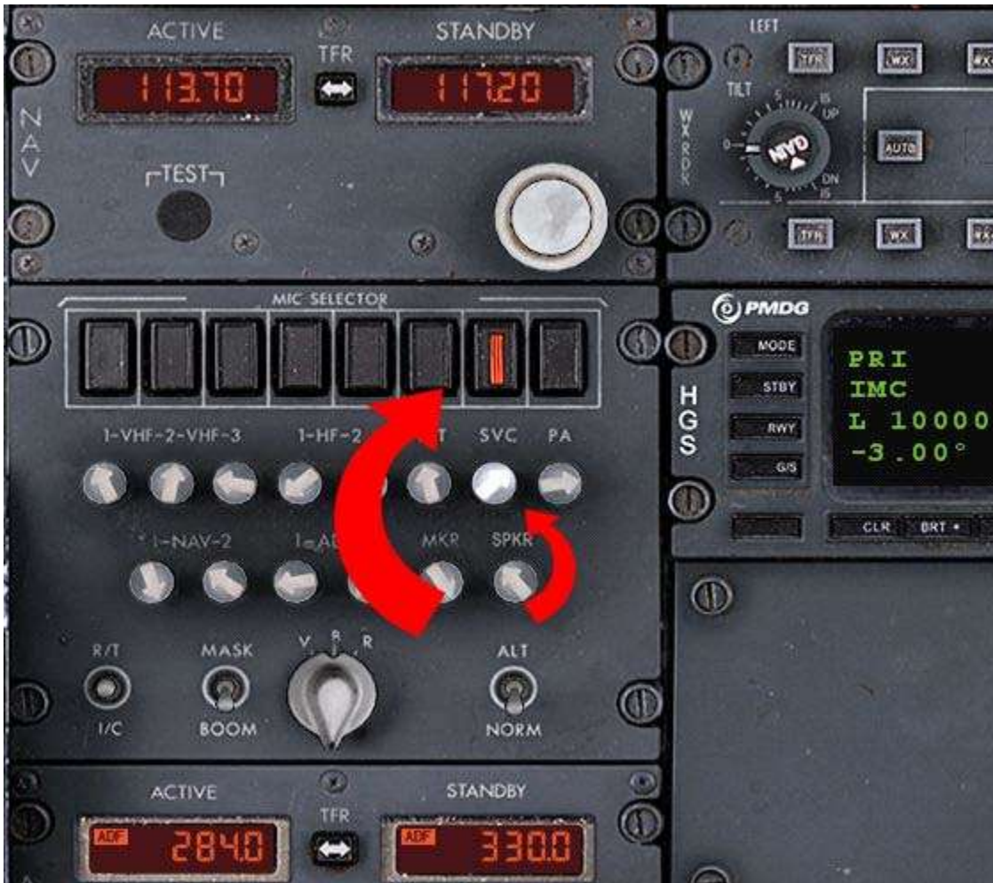
CAPTAIN'S AUDIO CONTROL PANEL - ENSURE 'SVC' IS PRESSED IN AND THE VOLUME IS UP
